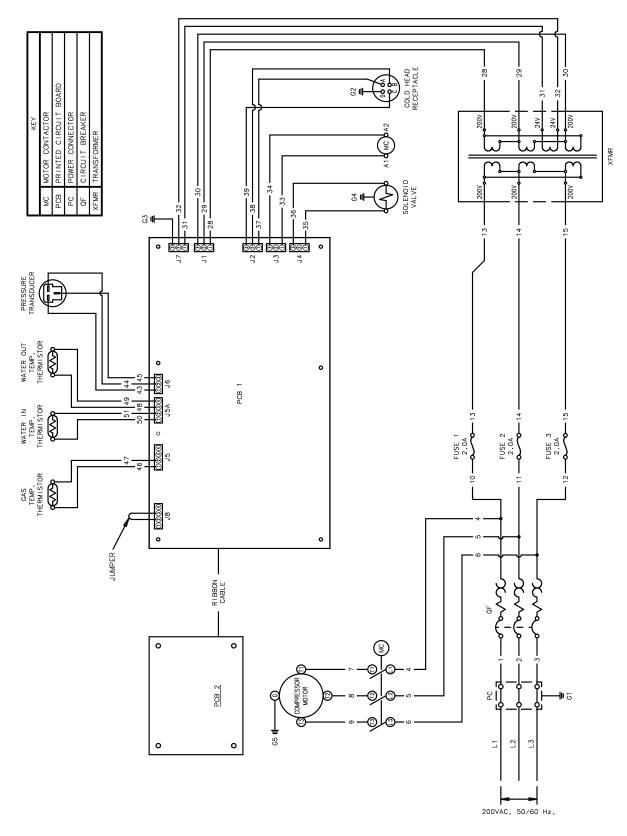
Figure 18 F-70L Compressor Wiring Schematic
