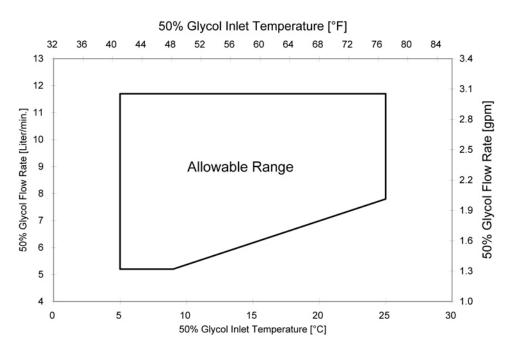
Figure 3 Allowable Glycol/Water Range for F-70 Compressor
