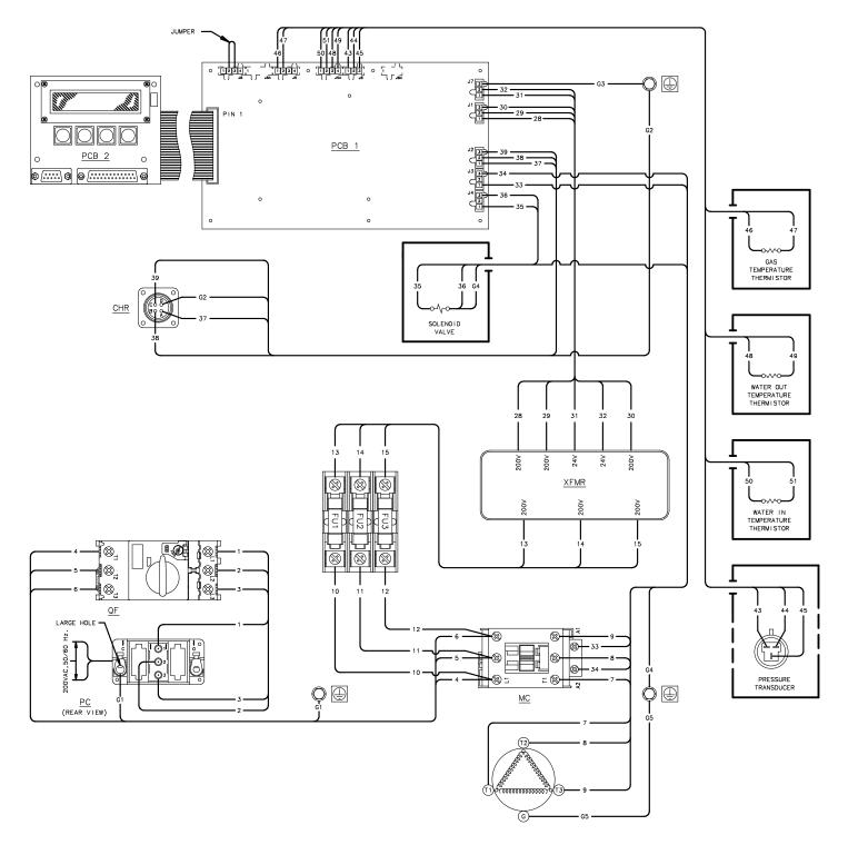
Figure 17 F-70L Compressor Wiring Diagram
