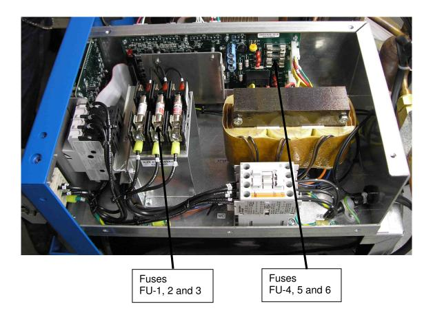
Figure 6 Fuse Locations in the Electrical Chassis
