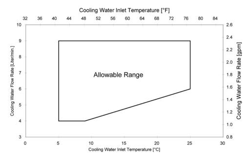
Figure 2 Allowable Cooling Water Range for F-70 Compressor
