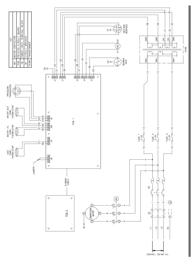
Figure 20 F-70LP Compressor Wiring Schematic
