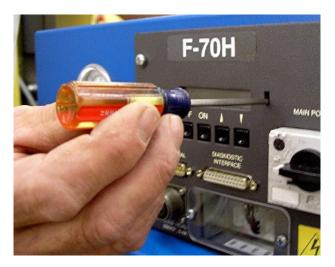
Figure 14 Set the Configuration Mode Selector Switch
