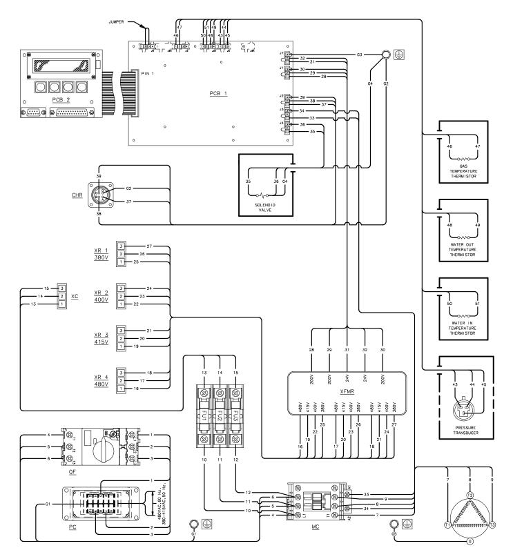
Figure 15 F-70H Compressor Wiring Diagram
