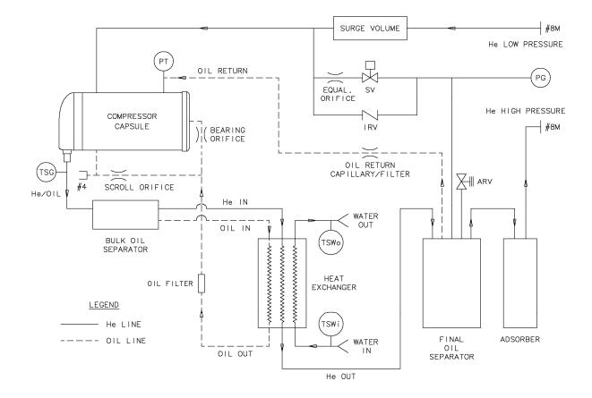
Figure 1 Compressor Flow Diagram
