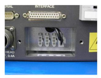
Figure 7 Voltage Selection Connectors
