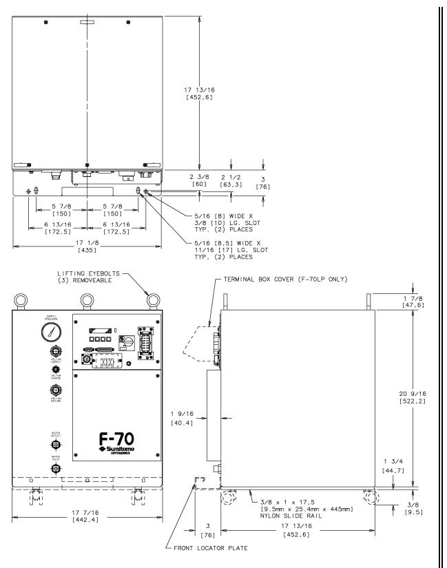
Figure 5 F-70H, F-70L and F-70LP Compressors, Dimensions
