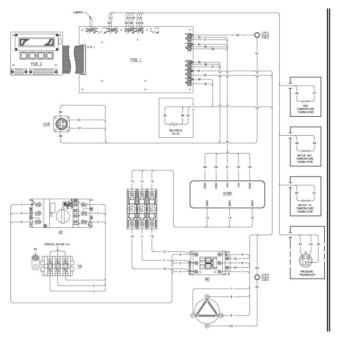
Figure 19 F-70LP Compressor Wiring Diagram
